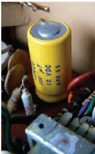
Figure 14.25 A capacitor (with a capacitance of 500 μF)
