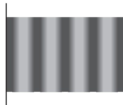
Figure 19.68 Equal thickness fringes for a wedge of equal inclination
