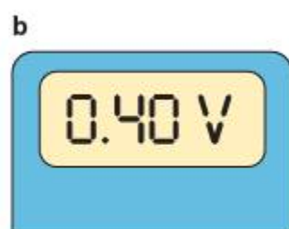
Figure 14.4 Two different voltmeters reading the same value of potential difference: a analogue voltmeter b digital voltmeter
