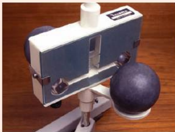
Figure 6.7 A modern version Cavendish's apparatus
