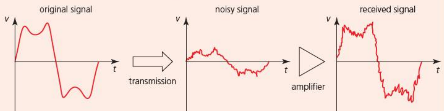
Figure 14.23 Amplification of a 'noisy' analogue signal
