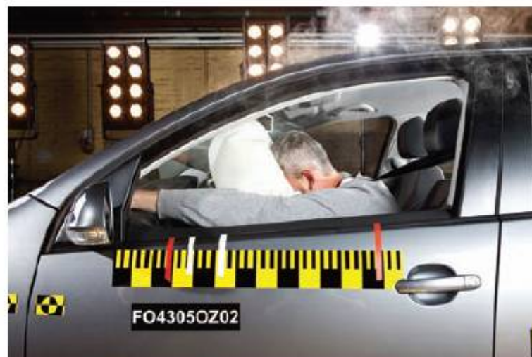
Figure 2.105 An air bag greatly reduces the forces in an accident
