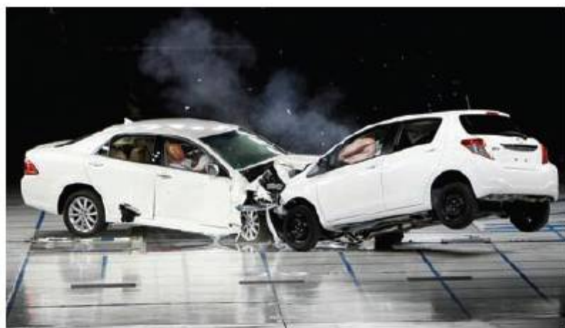
Figure 2.73 Momentum is conserved in this collision test
