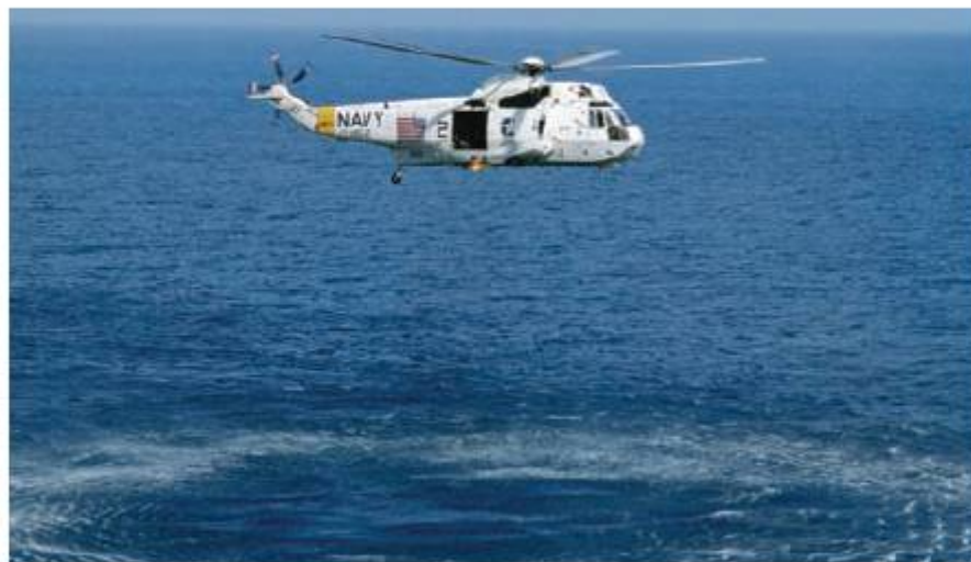
Figure 2.81 Helicopter blades give downwards momentum to the air
