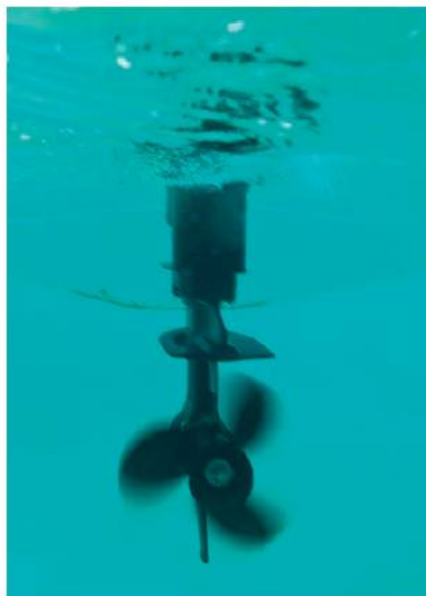
Figure 2.80 The propeller at the back of a boat exerts a force on the water and the water pushes back
