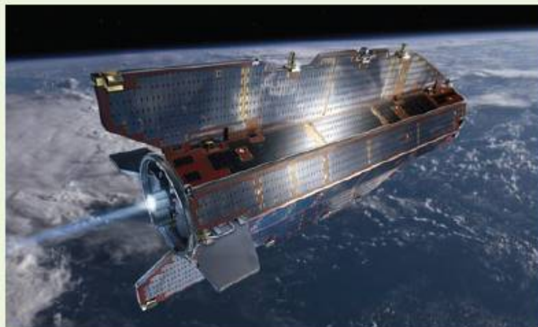
Figure 2.5 The Gravity Field and Steady-State Ocean Circulation Explorer (GOCE) satellite was launched by the European Space Agency in 2009 to measure the Earth's gravitational field in great detail
