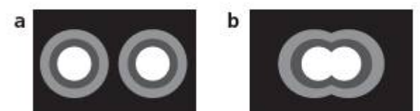
Figure 11.31 Images of two point sources observed through circular apertures that are a easily resolvable and b just resolvable
