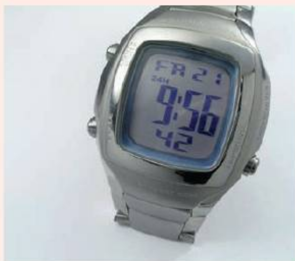
Figure 4.6 A digital watch relies on electrical oscillations
