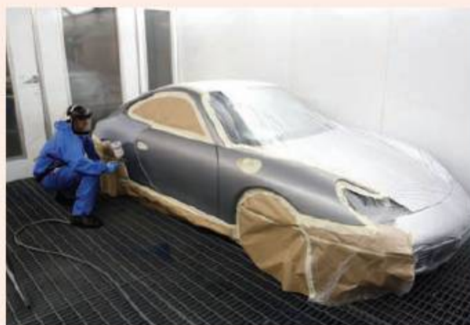
Figure 6.15 Electrostatic paint spraying ensures an even coating
