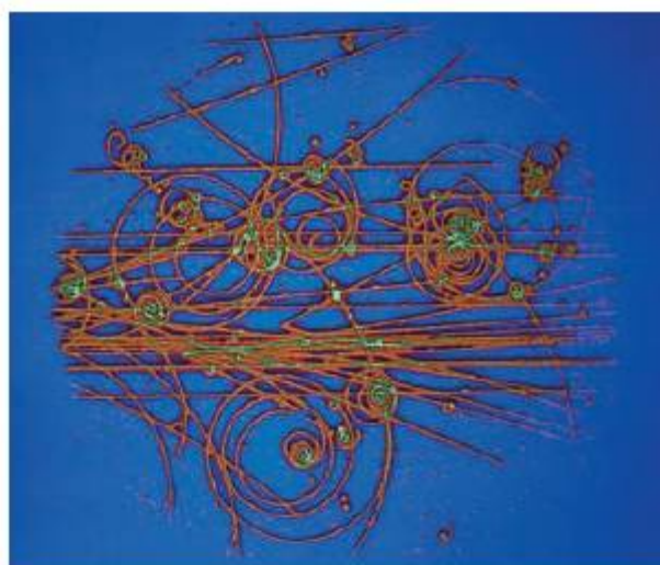
Figure 6.53 Curved paths of individual particles in a nuclear physics bubble chamber
