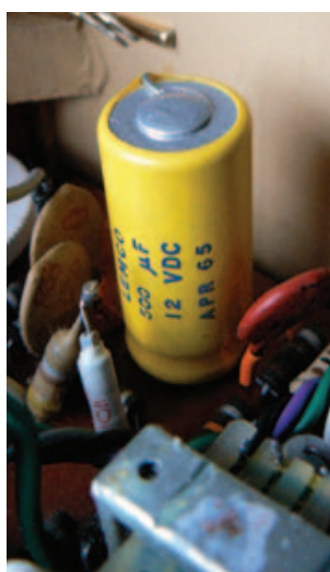
Figure 17.24 A capacitor (with a capacitance of 500 μF)
