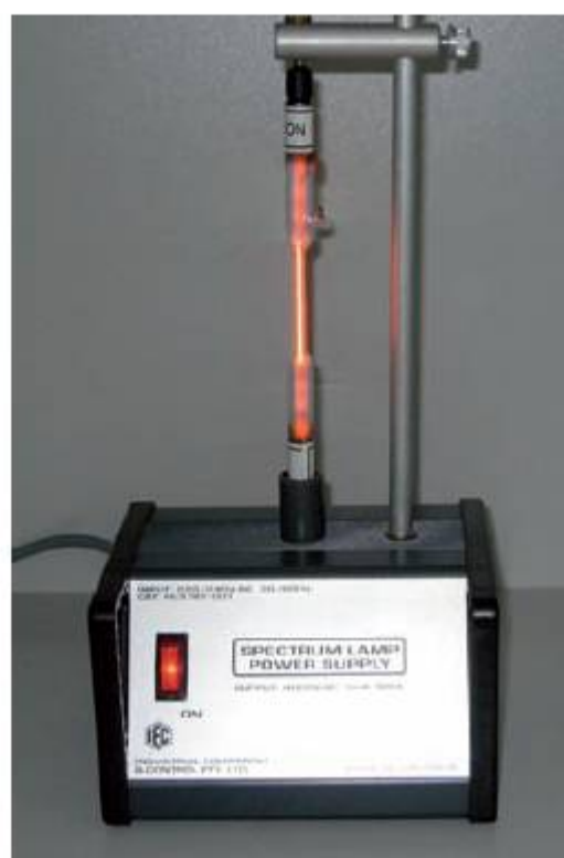
Figure 7.9 A discharge tube containing atoms of neon gas (at low pressure)
