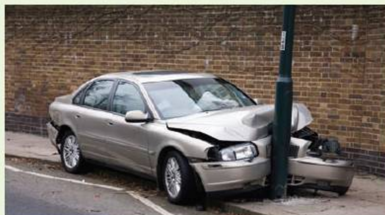
Figure 2.106 The front of the car is deformed but the passenger compartment is intact
