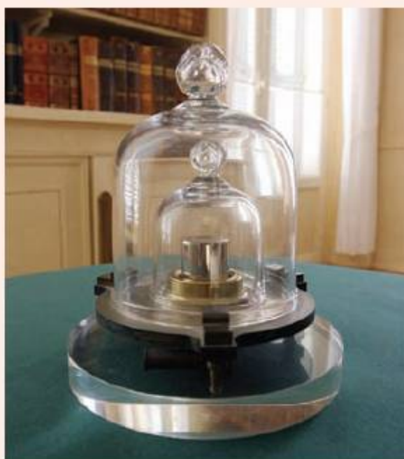
Figure 1.2 Replicas of the International Prototype Kilogram (IPK) are used across the world to act as mass standards. They are stored in air, in nested bell jars, and need periodic cleaning to remove atmospheric contamination
