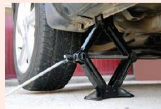
Figure 2.100 Changing a car tyre using a simple machine (car jack)
